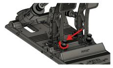
7. Adjust the pushrod length by turning the clevis until it approximately matches up with the hole in the pedal arm. Re-insert the clevis lock pin.
