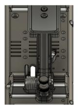
When installing your pedals, you will find that the USB Type-C female connector is pointing towards the throttle, not towards the pedal set's rear. This was a very intentional choice on our side to make sure you will not coincidentally break the connector. Note also the small cable clip on the top of the cover. We want to make sure that your cable is not strained and suggest you use the provided clip to alleviate any potential strain on the cable.
