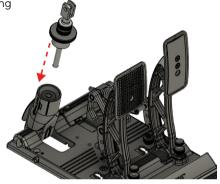
8. Re-insert the clevis lock pin.
