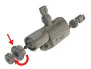
6. Grab the small thumbnut and turn it onto the shaft clockwise until it locks the larger thumbnut in place.
