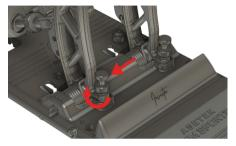
Adjust the pushrod length by turning the clevis until it perfectly matches up with the hole in the pedal arm.
