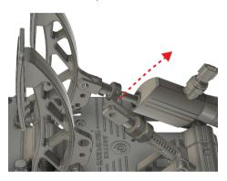
3. Remove the rod with spring from the pivot bracket.
