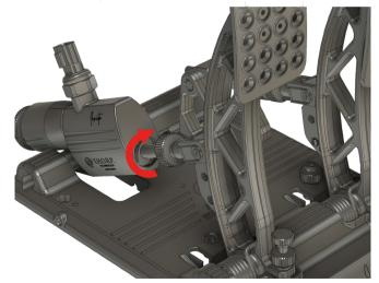
2. Remove the clevis lock pin
