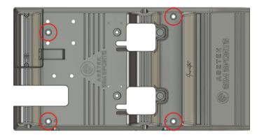
The baseplate is designed to be used with M6 screws, and holes in your rig should be with  $\emptyset$ 6,4 diameter. It is also compatible with the included M6 slot nuts
