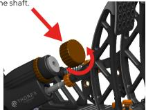
3. Press on the brake pedal with your hand until the elastomer with elastomer guide is visible. You can now take the elastomer with the elastomer guide out with ease.
