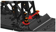
Adjust the pushrod length by turning the clevis until it perfectly matches up with the hole in the pedal arm.
