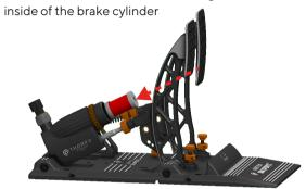
Grab the cylinder cap and screw it onto the brake cylinder clockwise, until you can feel light resistance from the top of the elastomer.
