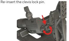
This way, there is no preload on the brake cylinder, which is essential to achieve a 100% stable calibration and not prematurely wear out the brake cylinder. Once these steps are completed, you should recalibrate.
