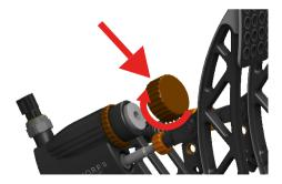
8. Tighten the orange lock nut on the most outer part of the brake cylinder by rotating it counter-clockwise to brake cylinder cap.
