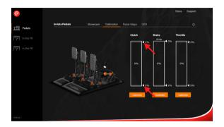
We suggest the following settings for deadzone when using the Asetek SimSports<sup>®</sup> Invicta<sup> $\mathsf{M}$ </sup> S-Series T.H.O.R.P. $\mathsf{M}$  II., which is how it is calibrated from our factory.
