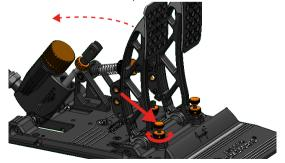
6. Tighten the locking thumbnut on the brake adjustment screw clockwise to secure it.
