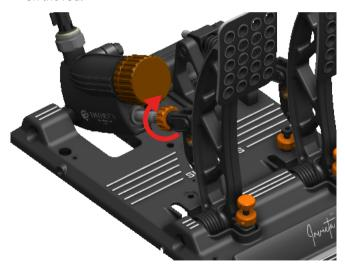
2. Remove the clevis lock pin. Push the Rod clevis lock pin upward to detach the pedal arm from the rod clevis and pull the pin outwards.
