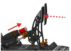
Take of the elastomer guide from both the top and bottom of the elastomer
