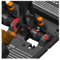
3. Swing the pedal rod out of the way.
