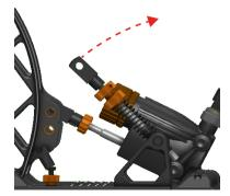
3. Push the pedal slightly forward, and rotate the thumbscrew (Clockwise to move the pedal forwards, Counter-Clockwise to move the pedal backwards)
