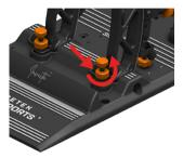
2. Remove the rod clevis and lift up the rod.
