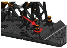
5. Push the pedal slightly forward, <u>and</u> rotate the thumbscrew
