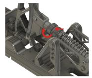
2. Remove the spring locking pins.
