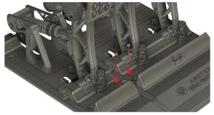
9. Route the cable under the Invicta<sup>™</sup> Brake & Throttle through the bezel and insert the cable to the Invicta<sup>™</sup> Clutch
