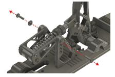
4. Align the clutch tension spring to the desired hole in the pivot bracket.
