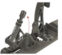
3. Unscrew the four screws underneath the clutch baseplate.
