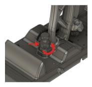
2. Push the pedal slightly forward, and rotate the thumbscrew (Clockwise to move the pedal forwards, counterclockwise to move the pedal backwards)
