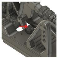
3. Re-tighten the thumbnut by rotating it clockwise.
