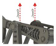
3. Remove the clutch pivot pin and bushing to release the clutch tension spring.
