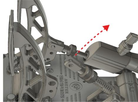
3. Remove the rod with spring from the pivot bracket.
