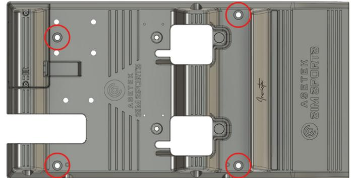
The baseplate is designed to be used with M6 screws, and holes in your rig should be with  $\varnothing 6,4$  diameter. It is also compatible with the included M6 slot nuts.
