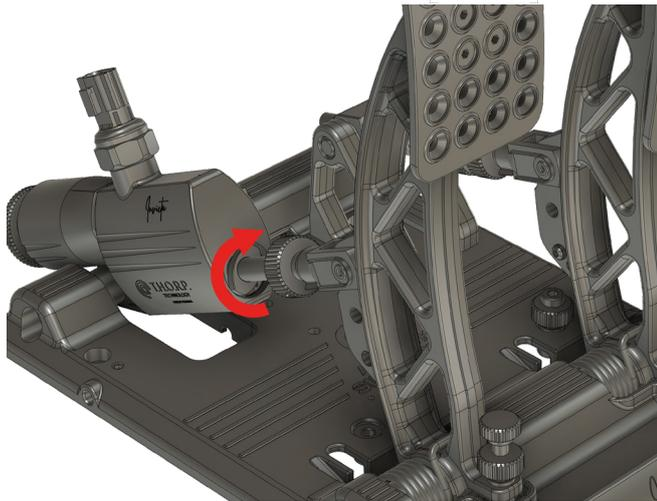
2. Remove the clevis lock pin
