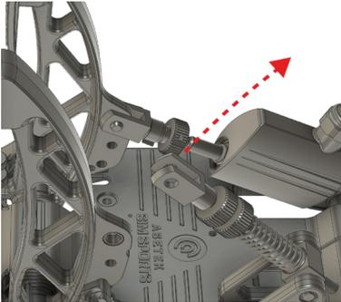
3. Push the pedal slightly forward, and rotate the thumbscrew (Clockwise to move the pedal forwards, Counter-Clockwise to move the pedal backwards)
