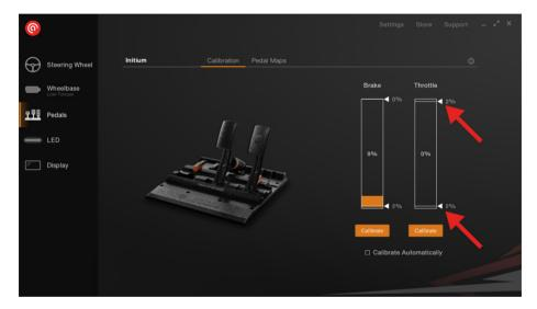
We suggest the following settings for deadzone when using the pedals, which is how it is calibrated from our factory.
