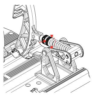
${\it 3. } \ {\it Turn the upper most thumbnut counterclockwise to retighten it,}$ locking the bottom thumbscrew in its position.
