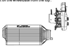
To Detach the wheel from an Asetek wheelbase, press the paddle on the wheels Quick Release adapter and pull the wheel up.
