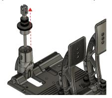
5. Carefully remove the elastomer with your fingers. If you cannot get it out with your fingers, use the pushrod spring to pull it out.
