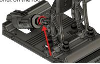
2. Remove the clevis lock pin
