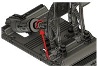
2. Remove the clevis lock pin.
