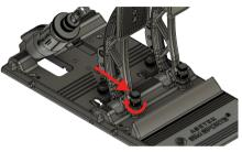
7. Adjust the pushrod length by turning the clevis until it approximately matches up with the hole in the pedal arm. Re-insert the clevis lock pin.
